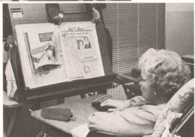
A patient, entirely paralysed below the neck, can control all the electrically-powered facilities in his room simply by applying pressure to a 'thin-pad', which in turn operates a 'Possum' control panel.
