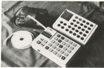
A Canon Communicator which produces a message on paper tape much in use by patients with speech difficulties.
