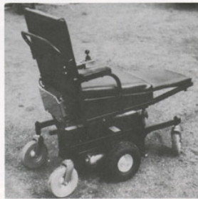
The electrically powered wheel-chair with power elevating seat, head-rest and foot-rest, designed by Mr. Eric Booth.
